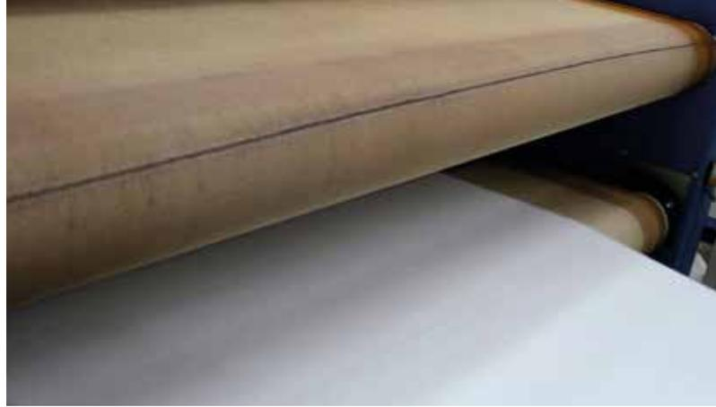
Glass hybrid belt with non-marking pin seam
