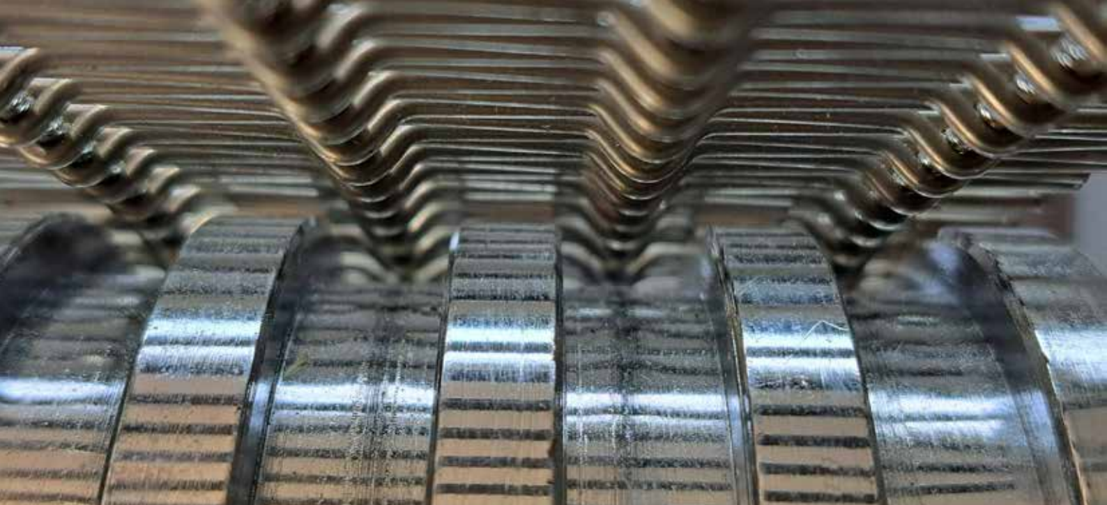
TRACKMATIC™ belt on grooved roller, ridge in the center (even number of V-crimps)
