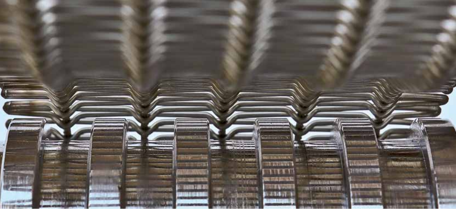
TRACKMATIC™ belt on grooved roller, groove in the center (uneven number of V-crimps)
