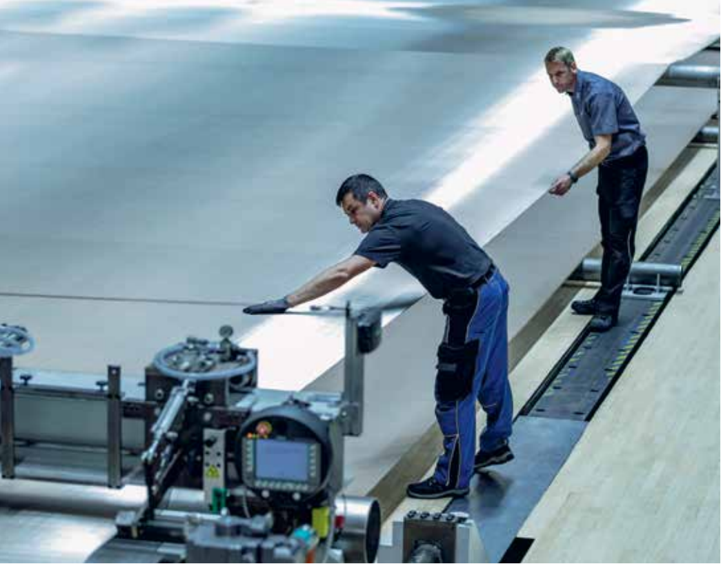
1. Pressing/embossing belt on the GKD stretching bench 2. Embossed OSB board 3. Diagram of a continuous press
